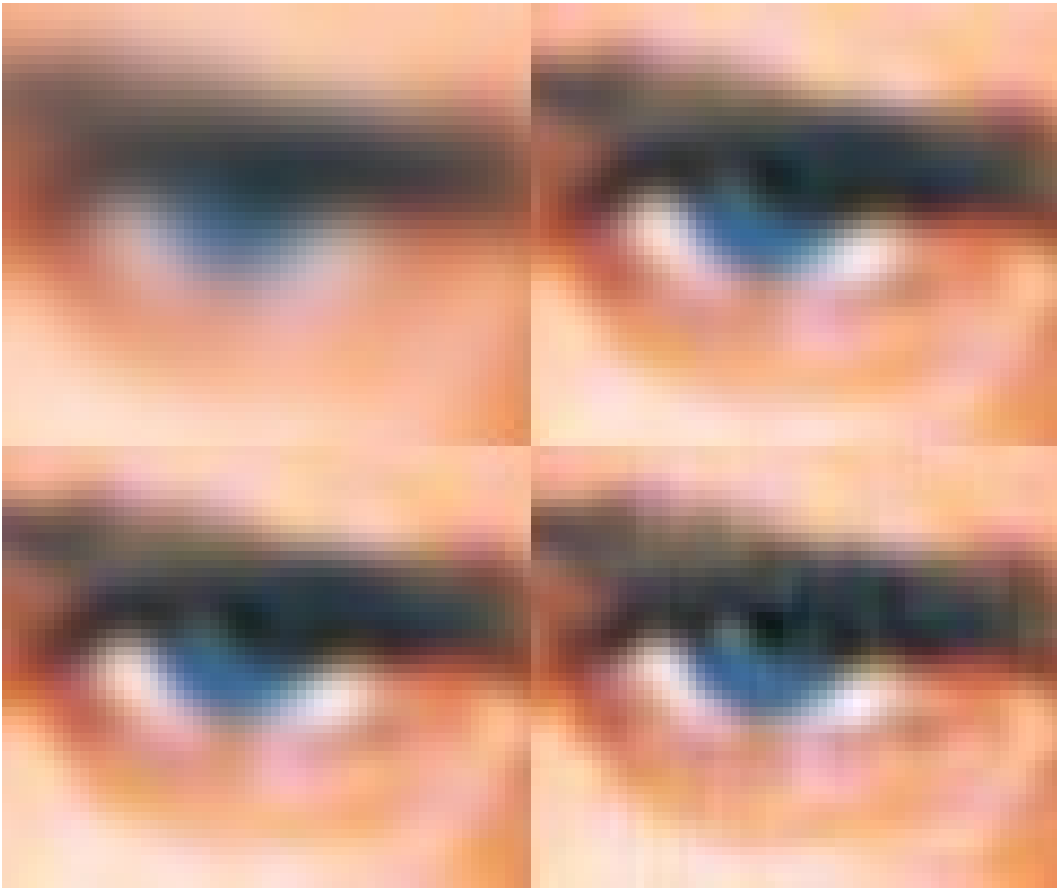
FIGURE 2. UL: input image. UR: Gradient descent. LL: ISTA, LR: FISTA. (200 iterations each)
